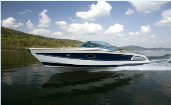
Electric battery-powered motor yachts: aquawatt 848 and boats with speeds of up to 28 knots
