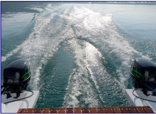
Power- Catamaran with double 13 kw outboard
