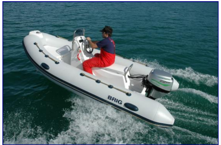
Falcon F 400 RIB with 13 kw engine, LI- batt. 19 knots speed
